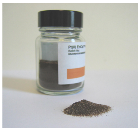
The spherical nature of Pt(0) EnCat™ makes it ideally suited to continuous flow processes or batch methodologies
